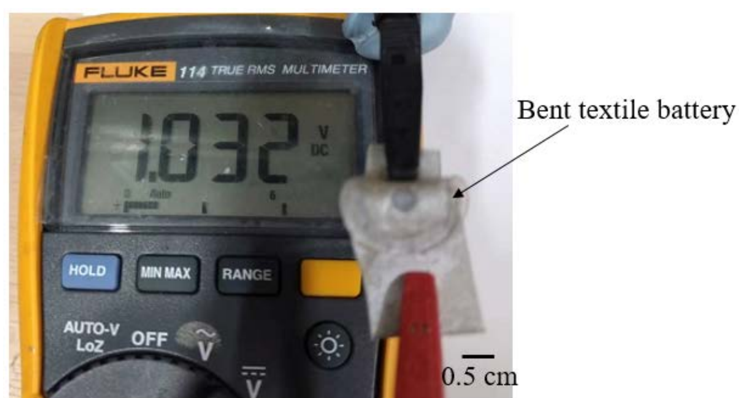
Figure 3. Battery initial voltage reading after encapsulation under 90 degree bending
