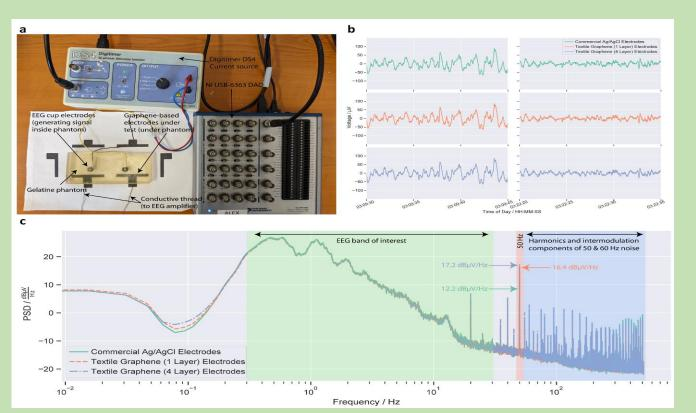
Printed graphene e-textiles for EEG applications. a) Experimental setup, b) Data collected using the textile graphene-based electrodes against commercial Ag/AgCl electrodes, c) Power spectral density of recorded signal from graphene textiles electrodes against commercial Ag/AgCl electrodes, highlighting the typical frequency band of interest in EEG studies shaded in green, higher frequency harmonics and intermodulation components from 50 and 60 Hz noise shaded in dark blue.
