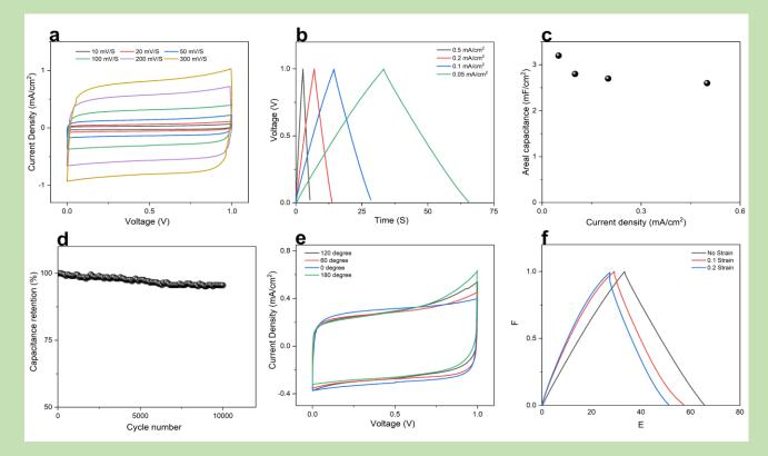
Characterization of graphene-based ink printed textile supercapacitor: a. CV curves at multiple scan rates, b. Charge/discharge curves at various current densities, c. The change of the areal capacitance with the current density, d. The cyclic stability of the printed supercapacitor measured at 0.1 mA cm<sup>-1</sup>, e. CV of the printed supercapacitor at different bending angles, f. Charge/discharge profile for the supercapacitor with no strain and under strain.
