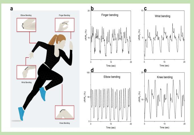
Printed graphene e-textiles as Piezoresistive activity monitoring sensors. a) Schematic diagram showing the application of graphene-based ink printed textiles as activity monitoring sensors at different body parts. The motion detection represented by the change of resistance as a function of time during b) finger joint bending c) wrist joint bending d) elbow joint bending and e) knee joint bending by the graphene-based ink printed textiles.
