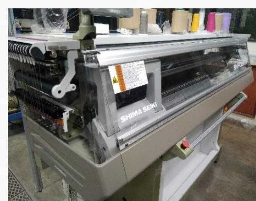
Shima Seiki V-bed knitting machine (14 gauge)
