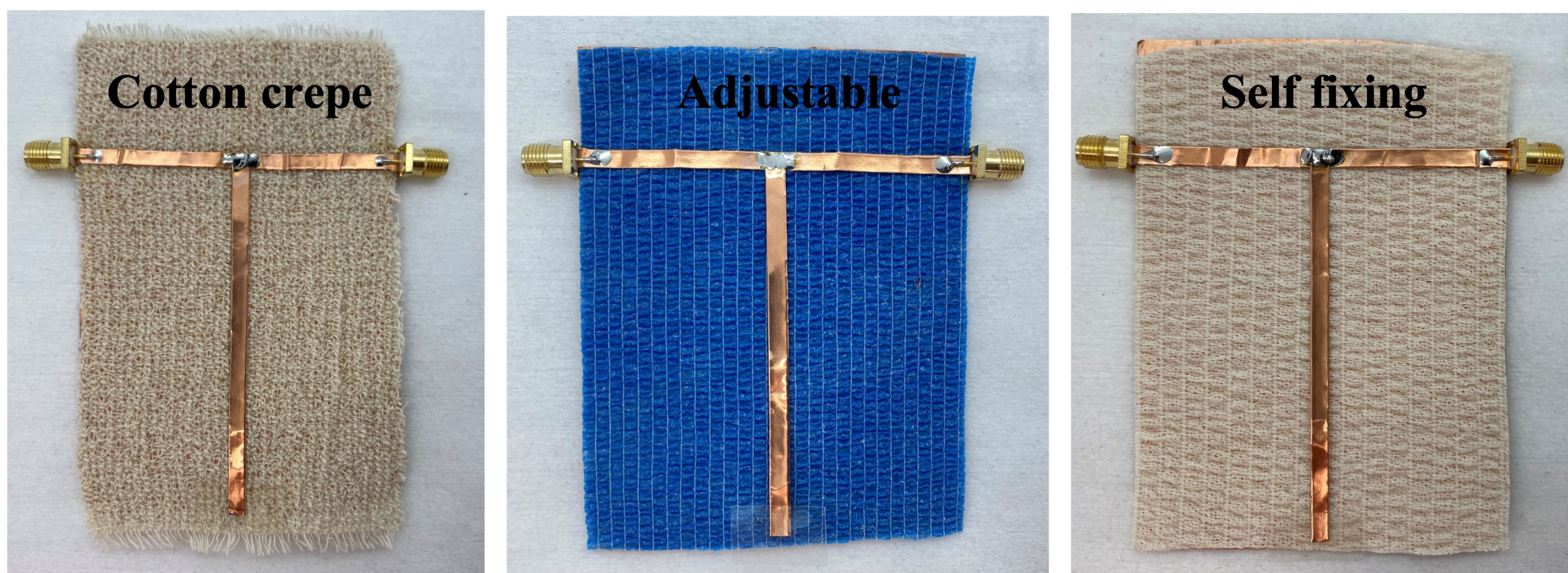
T-resonator designs for determining the relative permittivity of the bandage material
